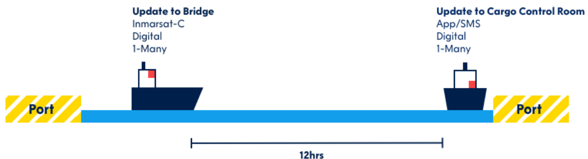
Figure 9: JIT using Inmarsat-C and App/SMS for communications
